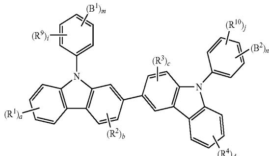
where:  $R^1$  to  $R^4$ ,  $R^9$  and  $R^{10}$  each independently represent a halogen atom, a substituted or unsubstituted alkyl group having 1 to 25 carbon atoms, a substituted or unsubstituted cycloalkyl group having 3 to 25 ring carbon atoms, a silyl group substituted by an alkyl group having 1 to 25 carbon atoms, or a cyano group;
