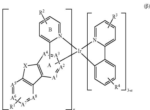
[0316] In the formula (β), A<sup>1</sup> to A<sup>8</sup> include a carbon atom or a nitrogen atom, at least one of A<sup>1</sup> to A<sup>8</sup> is a nitrogen atom, the ring B is bonded to the ring A by C—C bond, and iridium (Ir) is bonded to the ring A by Ir—C bond.
